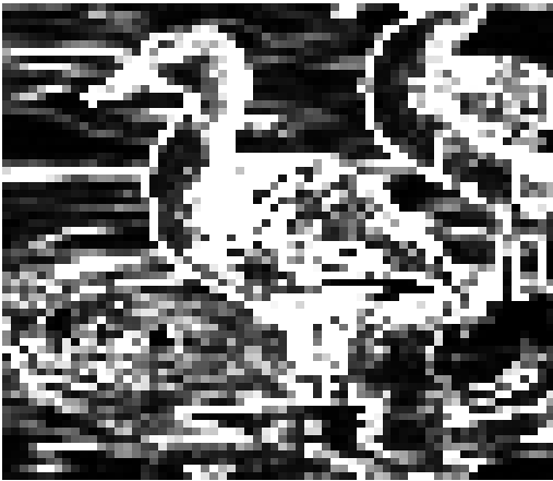
Figure 6: Variances of elementary blocks of the sample image. Higher values are represented by lighter regions. Note that variance values are inversely proportional to detectability.
